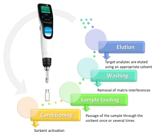
Figure 24. Different steps in MEPS procedure.
