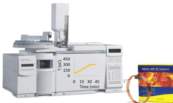
Figure 33. Agilent GC-MS equipment and temperature ramp used.
