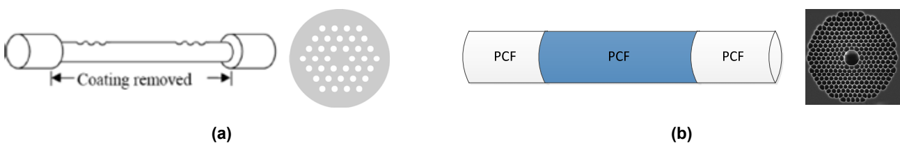
Figura 2.18 - Interferómetro (a) IG-PCF e (b) PBG-PCF [26]
