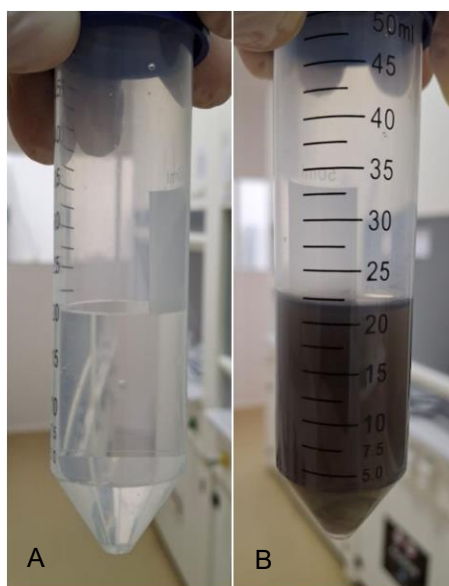
Figure 22. Color change in DA solution, before (A) and after (B) stirring for 3 hours.
