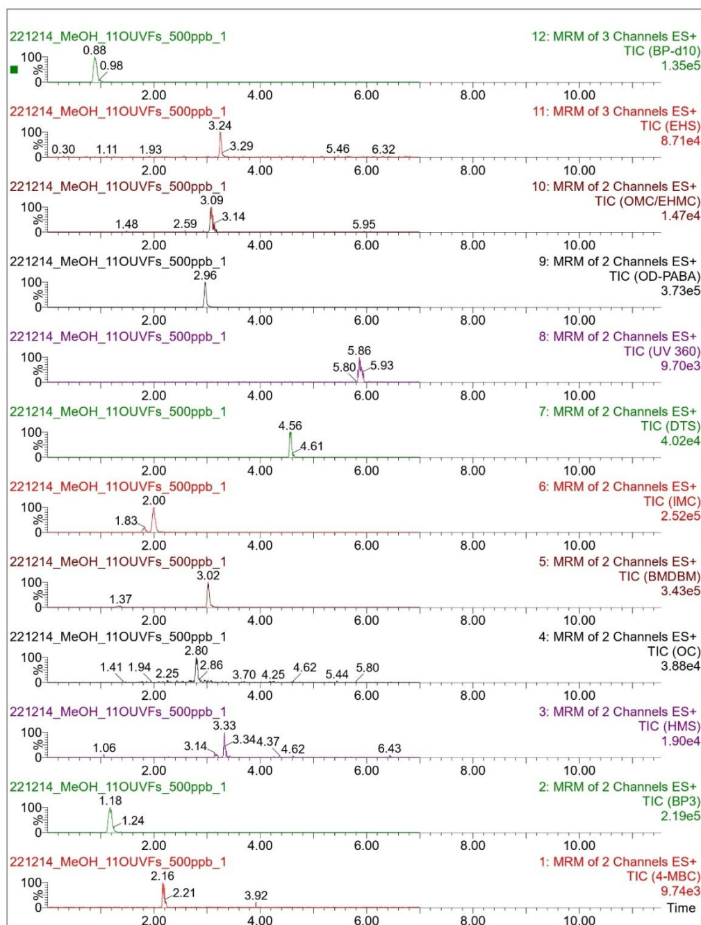
Fig. V. SM1. UHPLC-MS/MS chromatograms of the eleven target oUVFs and the internal standard (IS), BP-d 10 , at a concentration of 500 ug/L in methanol. Each panel represents a separate compound monitored using multiple reaction monitoring (MRM) in positive electrospray ionization (ES+) mode. The retention time (RT) for each compound is indicated by the peak apex in its corresponding trace.
