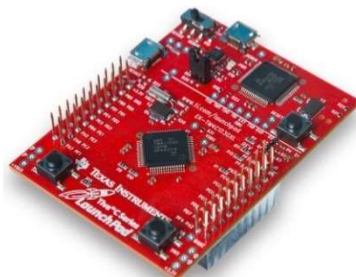
Figura 5.12 – Tiva C Series – TM4C123GXL launchpad .
