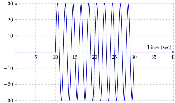
Figure 3.14: Signal generation for A_\theta = 30^\circ and f = 0.5 Hz
