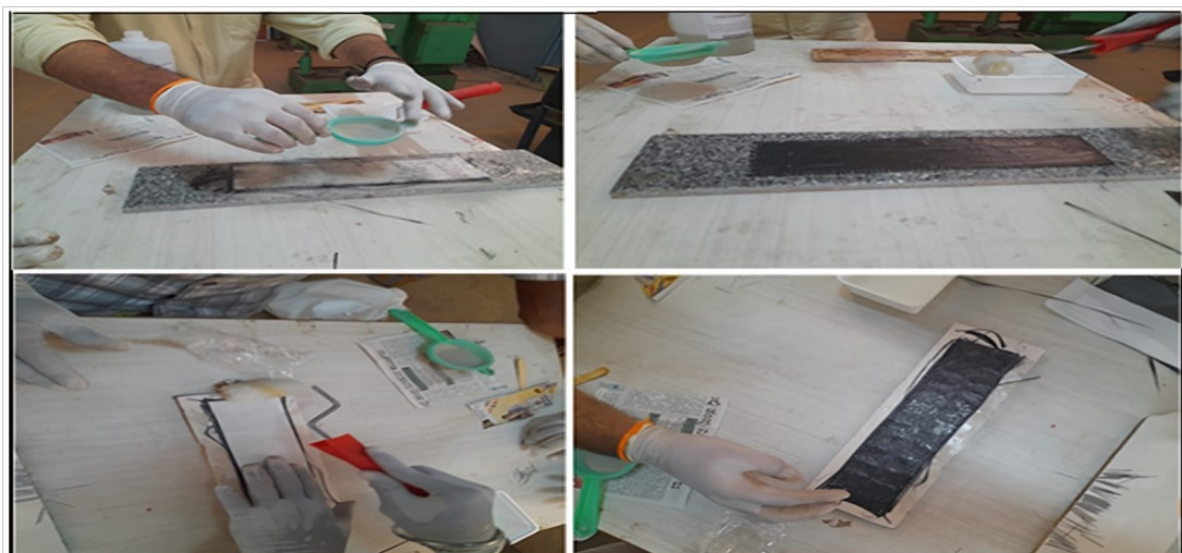
Figure 2. Fabrication of hybrid composites by hand lay-up technique.
