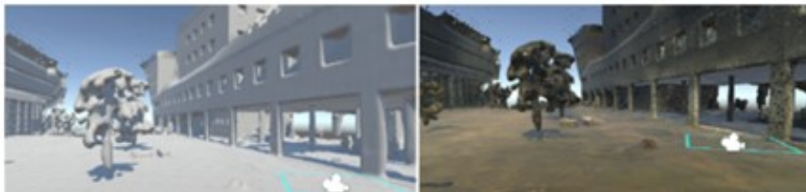
Figure 2.30: Importing the mesh as an as set into Unity: mesh with out colour information (left); coloured meshes with their respective textures (right) [31]
