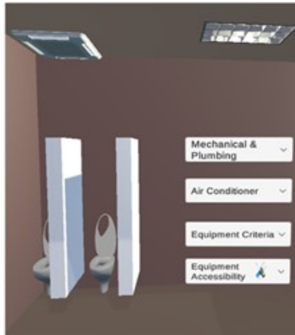
Figure 2.34: Automated checking of building component accessibility for maintenance in VR [5]- Inaccessible air conditioning system.
