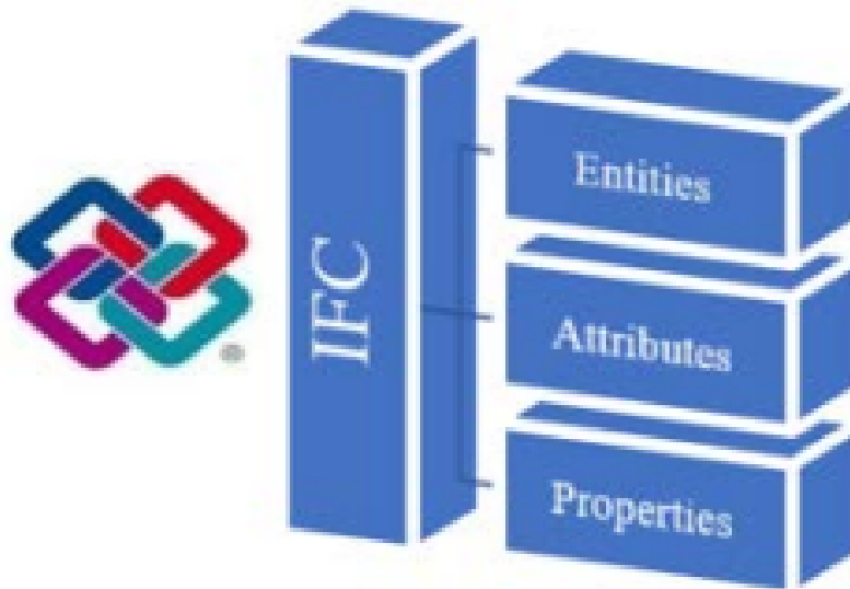
Figure 2.12: Basic IFC components [89]
