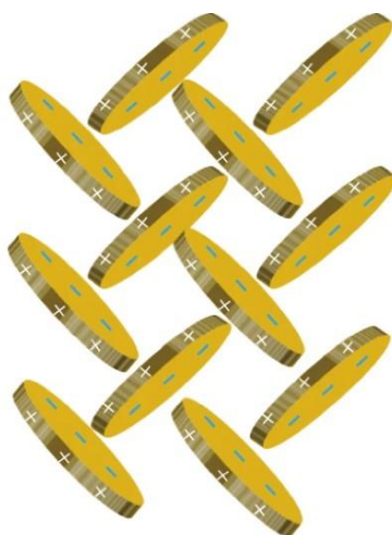
Figure 5 – House-of-Cards structure formed by electrostatic forces (47)
