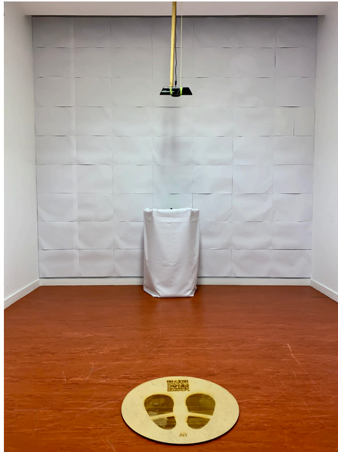
Fig. 9. Study setup with the Design Constraint, Kinect at 90^\circ relative to the floor, and a bin in a CAVE environment. A wooden stick supports the Kinect to provide stability since it is positioned far from the ceiling. The bin is hexagonal and made of Medium-Density Fiberboard (MDF) because it is easier and cheaper to replicate and is covered in a white cloth to optimize the projection from the projector. The wall is covered in several white A4 pieces of paper because it is painted gray, which could misrepresent the colors of the projection. Running along with the ceiling with adhesive putty from the Kinect to the computer is a single wire that later divides into 2 - one for power and another for data. The data wire from the Kinect is connected to an USB extension. This extension is then connected to a USB 2.0 to USB-C adapter and then to the computer. The DC on the floor is made of MDF with the feet pictogram, and it was recycled from another project, therefore the QR Code, which is irrelevant for this setup. The projector is behind the DC on its right, close to the ceiling on top of a cabinet. To increase visibility and produce brighter colors, we tapped every lab window with black cardboard.
