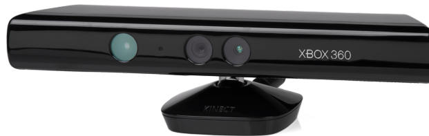
Fig. 11. The Microsoft Kinect v.1 [9] is equipped with an infrared sensor that can perceive depth. Since the floor is flat, if the litter is thrown to the ground, the infrared will detect a difference in depth and tell the computer to draw it on the depth image.
