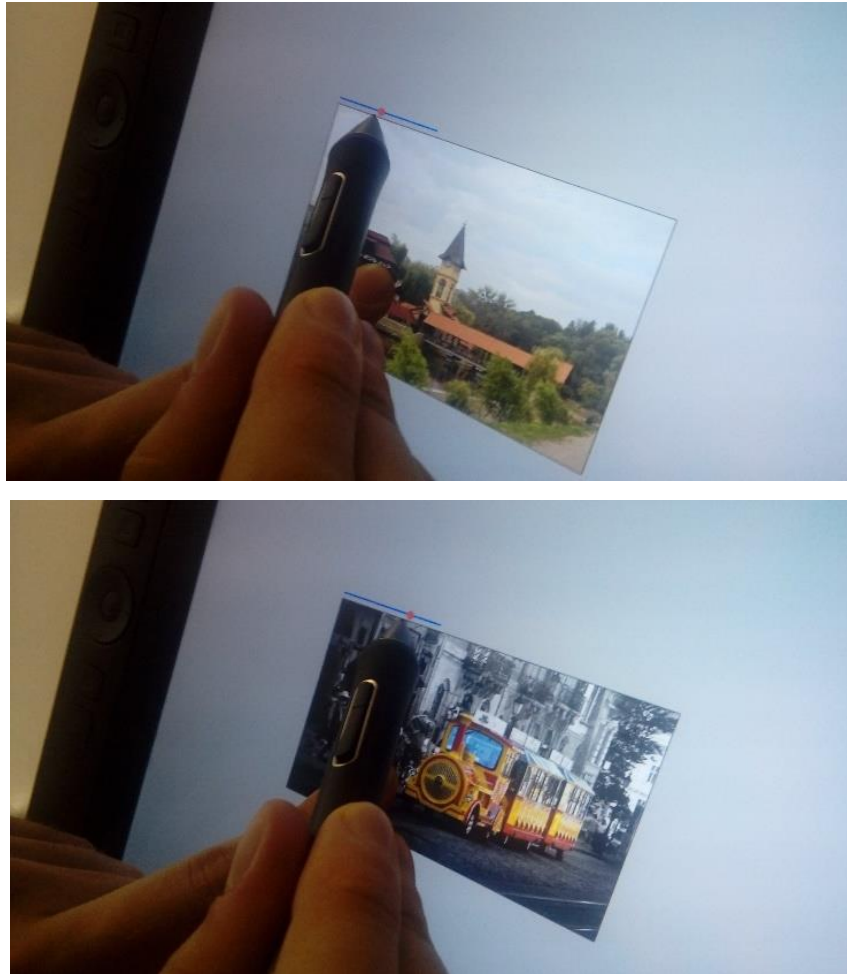
Figure 32. When holding a widget, users can move tiny slider using the pen to switch images.
