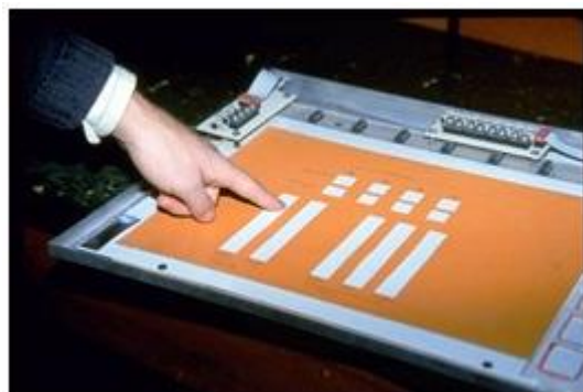
Figure 2. One of the first touch screens, invented by Bob Boie in 1984.
