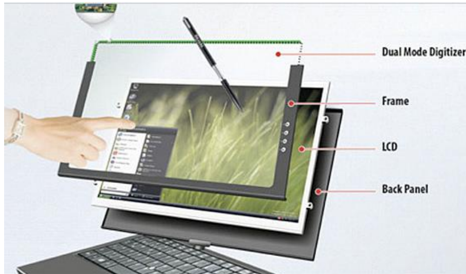
Figure 6. N-Trig, one of the modern non-Wacom pen and touch architectures.
