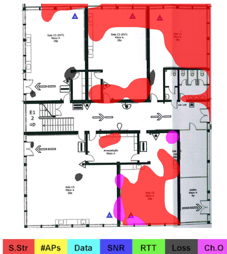
Figura 71 - Heatmap do Network Issues piso 0 Bloco C
