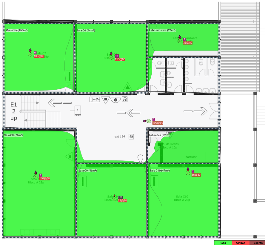
Figura 107 - Heatmap do Capacity Health piso 1 bloco C
