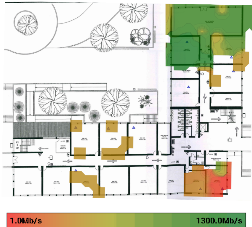
Figura 56 – Heatmap do Data Rate no piso 1 Bloco B
