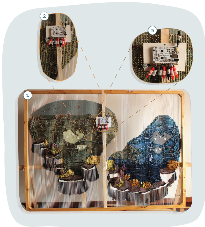
Fig. 36. Connections from the tapestry to the BCTB: (1) Back side of the interactive tapestry with the connections to the BCTB; (2) Conductive threads positioning; (3) Alligators connected to the BCTB.
