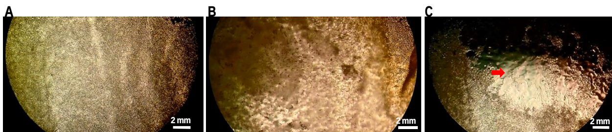
Figure 77 - Behaviour of a DNA/dendrimer film based on G5 PAMAM dendrimer (N/P ratio 4) under extreme pH changes. (A) Film without any solution, (B) after concentrated HCl addition (the film does not dissolve), (C) after concentrated NaOH addition (red arrow indicates immediate dissolution).
