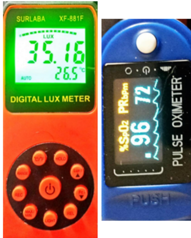
Figure.12: Lux meter (left) and CMS60C pulse oximeter (right) used for data collection.
