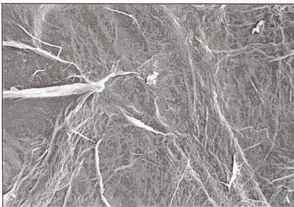
Fig. 3.(A) – SEM microphotograph of top surface of handsheets made of Dwarf Cavendish pseudo-stem: (A) \times 1500 ;
