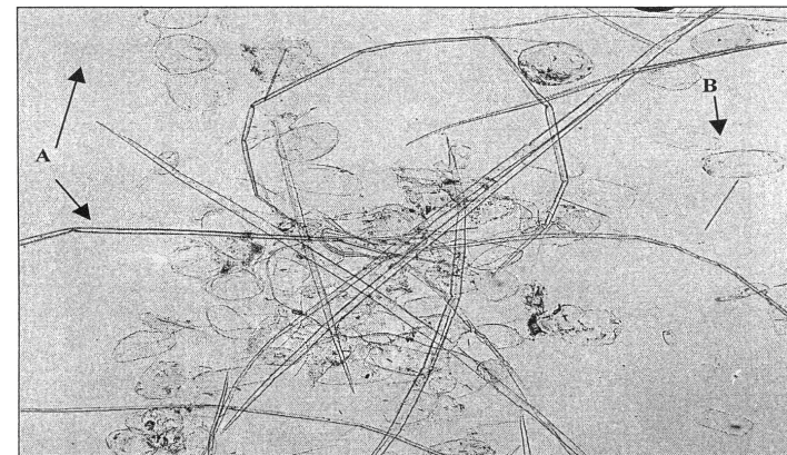
Fig. 2. – Micrograph (10X) of P_{120} pulp from Dwarf Cavendish pseudo-stem: (A) fibre and (B) ground tissue cell.
