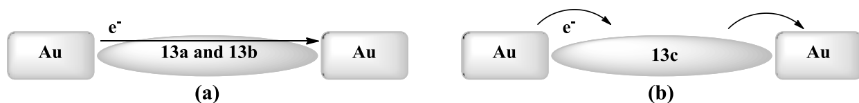
Scheme 3. Charge transport for the systems reported by Rigaut and co-workers at 5K: (a) direct tunnelling for 13a and 13b junctions, (b) sequential tunnelling for the 13c junction. Adapted from refs. [53f, 57].
