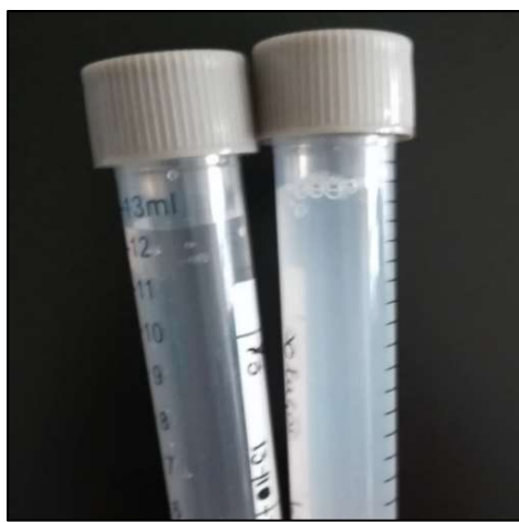
Figure 31 - Nanogel-0 (left) and Nanogel-20 (right) 1 hour after thawing. Note: The opacity of Nanogel-20 is reversed after 24 hours, with the solution returning to its original clear state.
