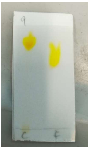
Figure 49 - Purification of the Alendronate-FITC conjugate by Thin layer chromatography on silica plate using as eluent a mix of tetrahydrofuran and methanol in 1:10 volume ratio. The conjugate was applied on the left side of the plates and FITC was applied on the right side.
