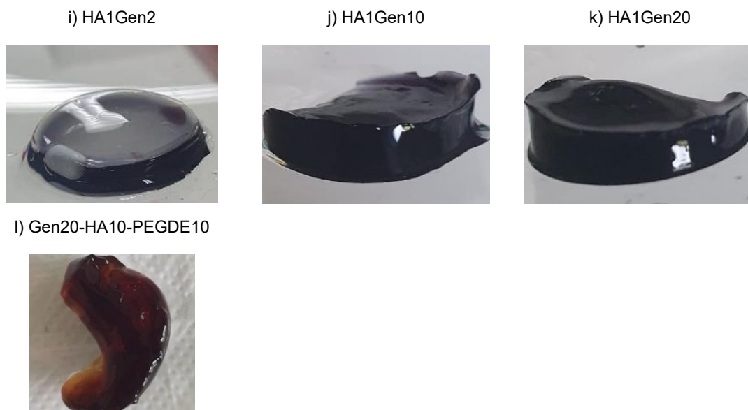
Figure 12 - HA-based hydrogels. HALys was used for HAGA, HA-Gen and Gen-HA-PEGDE hydrogels formation, meanwhile native HA (0.6-1.0 million Da) was used for the formation of HA-PEGDE and HA-EGDE hydrogels.
