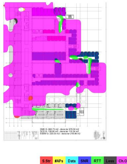
Figura 5.6-Network issues do piso 2
