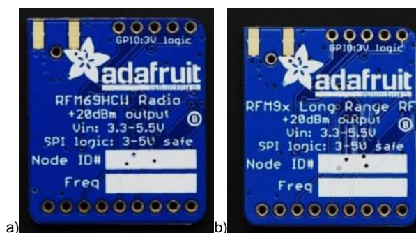
Figura 3.31 Módulos RF LoRa [65]: a) RFM69HCW. b) RFM9x LoRa [65].
